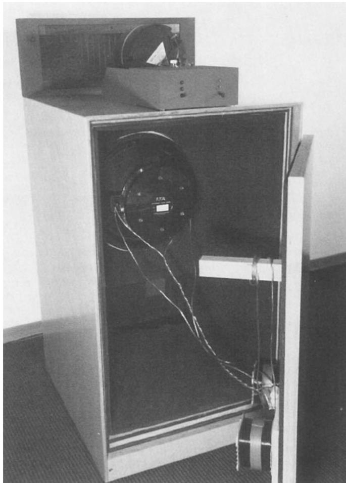
range. In addition to this, a Tractrix curve would allow a nice visual effect because the 45 degree angle of the cabinet walls blends perfectly with the miter joints we intended to use for the cabinets. According to Dinsdale's and Lambert's work, the true cutoff in a Tractrix horn occurs at the 70% to 80% point of the mouth area — the cabinet walls precisely made up for this percentage.
